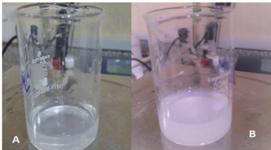
Figure (8-B) Synthesizing media(ISP4) (A): before and (B) after Biosynthesis of ZnO nanoparticles.
