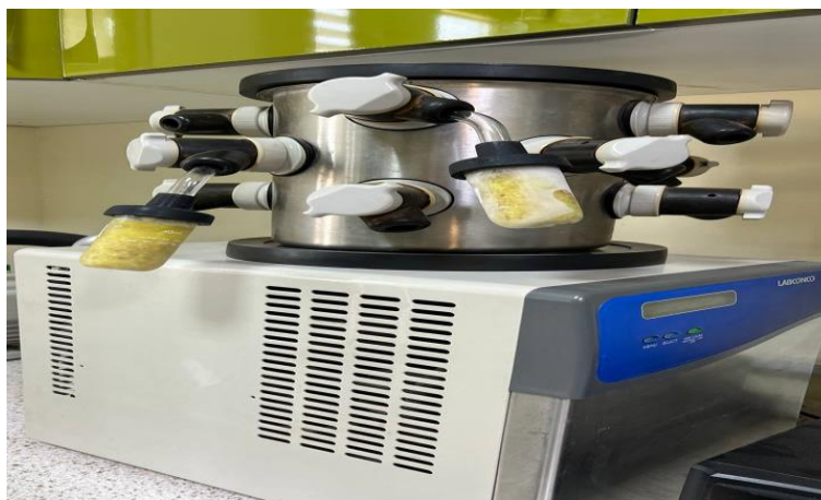
Figure 2.2: frozen crude ginger sample is connected to the freeze dryer
